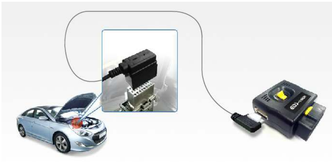
Fig. 8-4 CVCI : Connecting and using engine room 20-pin terminal
