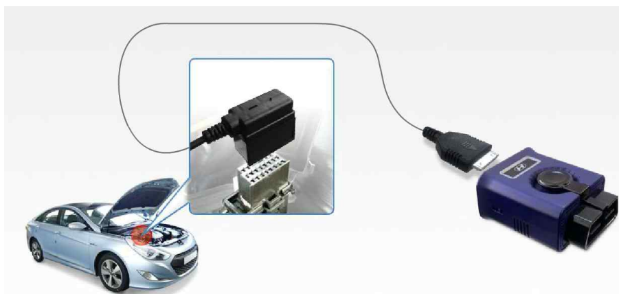
Fig. 8-5 VCI-II : Connecting and using engine room 20-pin terminal
