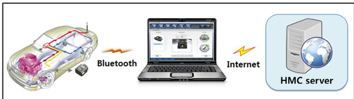
Fig. 3-1 Conceptual diagram of Smart DLogger communication
