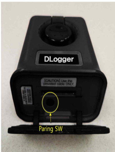
Fig. 3-10 CVCI-II Pairing switch
