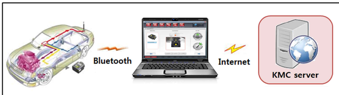
Fig. 3-1 Conceptual diagram of Smart DLogger communication
