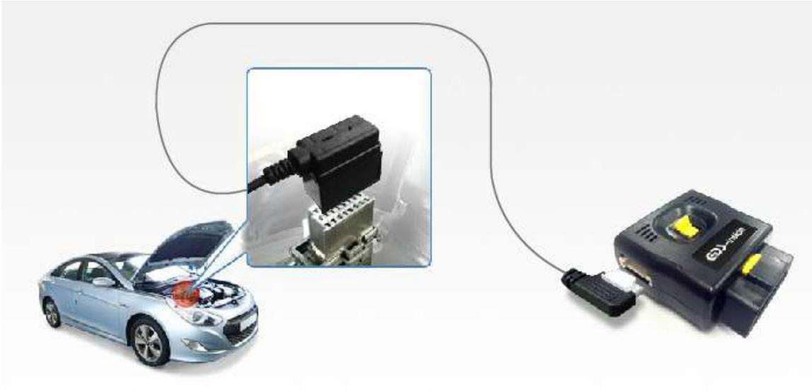
Fig. 8-5 CVCI : Connecting and using engine room 20-pin terminal – Method 2
