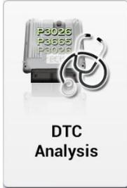
DTC Analysis is to retrieve DTC data from a specific ECU and retrieve diagnostic procedures for any DTCs found.
