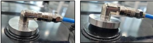
[Normal connection] [Abnormal connection]
