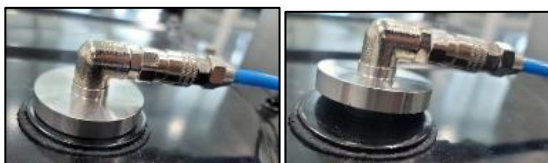
[Normal connection] [Abnormal connection]
